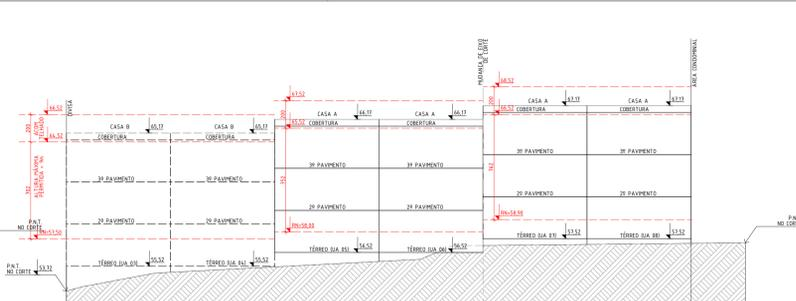
CORTE ESQUEMÁTICO D-D
